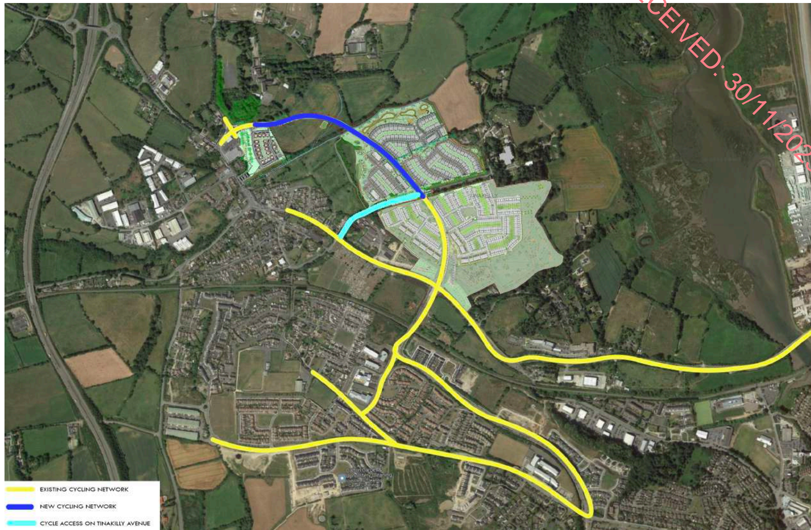
Figure 4 – Existing Cycle Network Integration with New Cycle Facilities and Cycle Access Through Tinakilly Avenue
